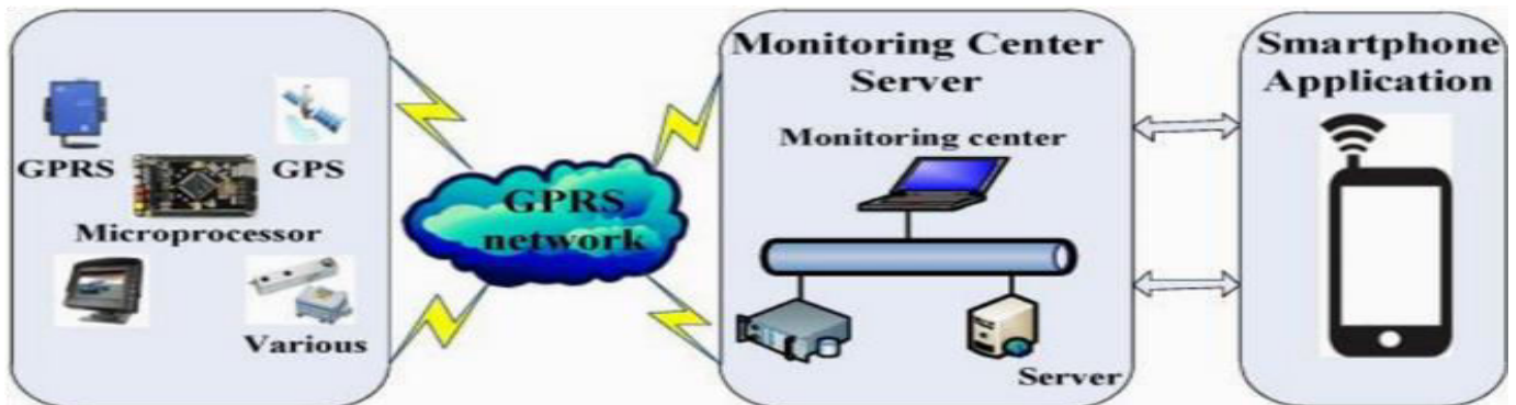
Figure 1: System Communication and Security.
